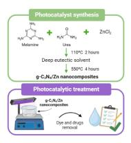
In recent years, there has been a growing interest in the use of environmentally friendly Deep Eutectic Solvents (DES) for the ecological synthesis of different nanoparticles. Their combination with Advanced Oxidation Processes (AOPs) for water treatment is emerging as a sustainable alternative to conventional methods.
