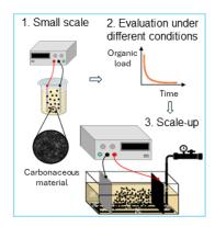
Conventional wastewater treatment processes have demostrated low efficiency in removing recalcitrant pollutants, characterized by high persistence and organic content. Adsorption and advanced oxidation processes have emerged as economical and sustainable techniques for reducing and/or eliminating the presence of these harmful organic compounds in polluted waters.
