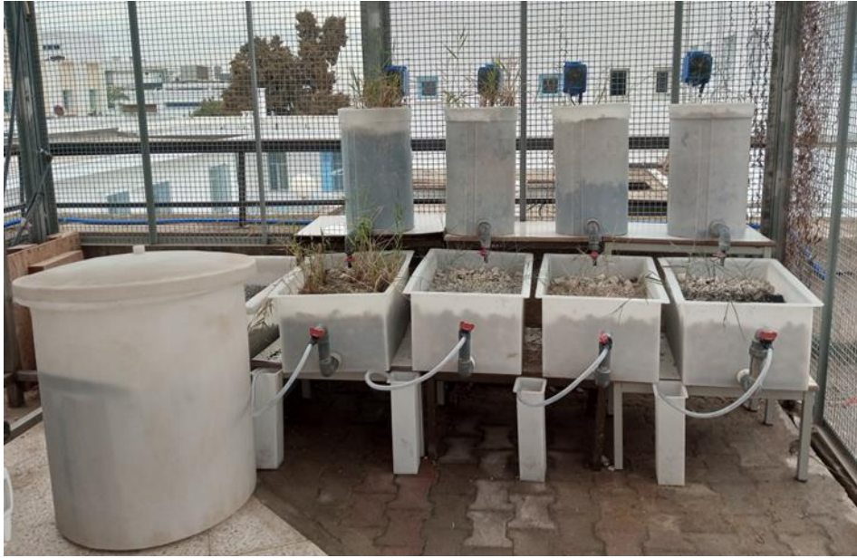
Figure 2.3.2.1 First lab-scale constructed wetlands.
